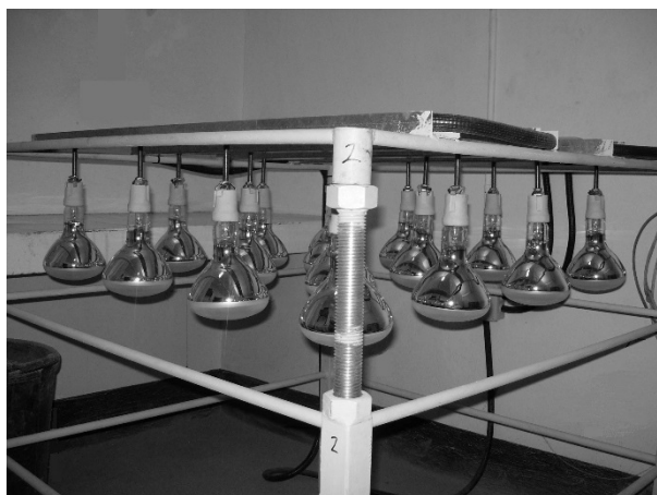
Fig. 3 - Solar simulator lamp used for the thermal (irradiation) tests of the asphalt slabs.
