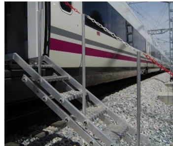
b) Evacuation to track level.
