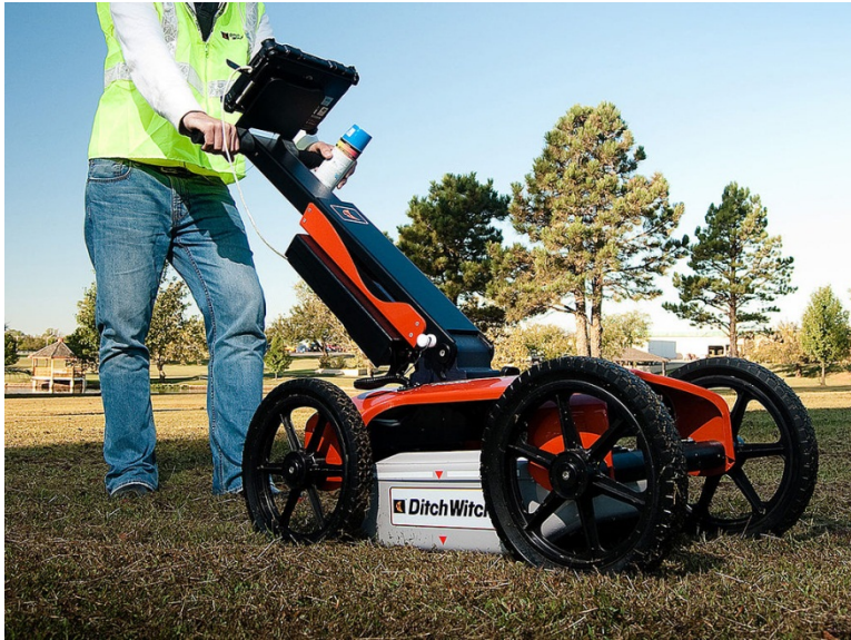
Fig. 28. GPR system in use [50]
