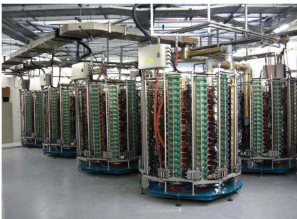
Fig. 12. 5-tower array of 40 kW per tower, 200 kW total CW power. Used with permission.
