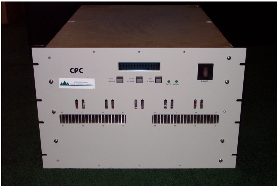
Fig. 4. High-efficiency amplifier for MRI. Courtesy of GMRR [11].
