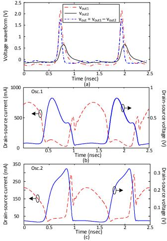
Fig. 7 Differential extraction of pulsed waveforms using a forcing AG in one of the oscillator elements. (a) Pulse sharpening with the second oscillator biased at  $V_{DD2} = 1.1$  V and phase shift  $\phi = 15^{\circ}$  (b). Drain voltage and current waveforms for first oscillator with
