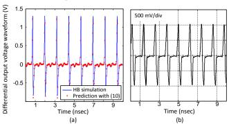
Fig. 12 Monocycle waveform obtained for  $V_{DD2} = 2.5$  V and  $\phi = 9.8^{\circ}$ . (a) HB simulation and prediction with (11). (b) Measurement.
