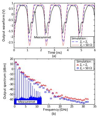
Fig. 3 Output signal of the NLTL. (a) Simulated and measured waveforms. The experimental waveform was obtained with the digital oscilloscope Agilent DSO90804A. (b) Spectra.
