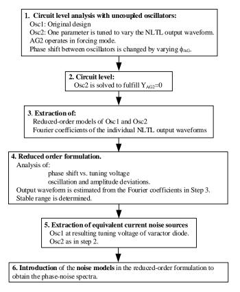
Fig. 6 Flow-chart indicating the steps to be taken for the design of the coupled system of two NLTL-based oscillators.
