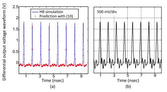
Fig. 11 Pulsed waveform obtained for  $V_{DD2} = 1.1$  V and  $\phi = 15^{\circ}$ . (a) HB simulation and prediction with (11). (b) Measured waveform.
