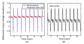
Fig. 13 Switched polarity monocycle obtained for  $V_{DD2} = 2.5$  V and  $\phi = -16^{\circ}$ . (a) HB simulation and prediction with (11). (b) Measurement.
