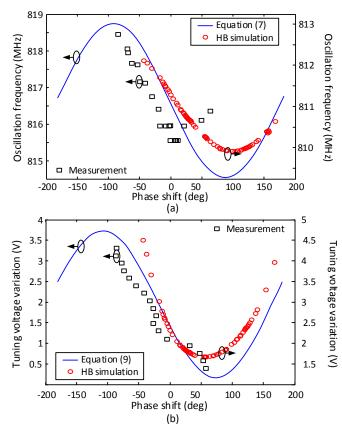
Fig. 9 Coupled system of two oscillators biased at  $V_{DD1} = 2.9$  V and  $V_{DD2} = 1.1$  V. (a) Oscillation frequency variation versus the phase shift, obtained with (8) and with HB. Measurements in the stable range are superimposed. (b) Tuning voltage variation versus the phase shift using (10) and HB. Measurements are superimposed.
