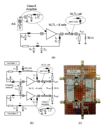
Fig. 4 NLTL-based coupled oscillator system. (a) Schematic of the individual oscillator. (b) Coupled oscillators. (c) Photograph.
