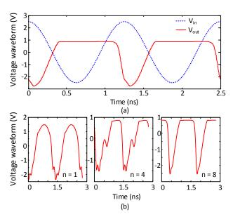
Fig. 2 NLTL with n = 8 and L = 0.3 nH. (a) Comparison between input and output voltage waveforms. (b) Waveform evolution though the NLTL cells.
