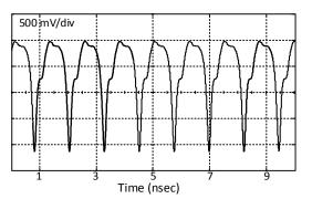
Fig. 5 Measured output signal of the sharpened–waveform oscillator terminated in 50  $\Omega$ .
