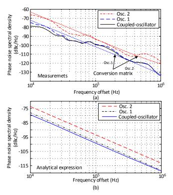
Fig. 15 Narrow pulse generator. (a) Phase noise spectral density of the two individual oscillators and the coupled system. Results of the conversion-matrix approach are compared with experimental measurements. (b) Predictions with the approximate formulation (24).
