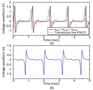
Fig 8 Monocycle waveform. (a) Parameters:  $V_{DD2} = 2.5$  V and  $\phi = 9.8^{\circ}$ . (b) Switched polarity monocycle with parameters:  $V_{DD2} = 2.5$  V and  $\phi = -16^{\circ}$ .
