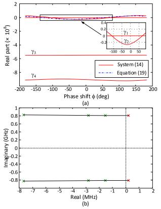
Fig. 14 Stability analysis of the coupled-oscillator system providing a narrow pulse. (a) Analysis versus the phase shift based on (15), with the result of the approximate expression (20) for  $\lambda_2$  superimposed. (b) Results of pole-zero identification at circuit level for the particular phase shift value  $\phi = 15^{\circ}$ .
