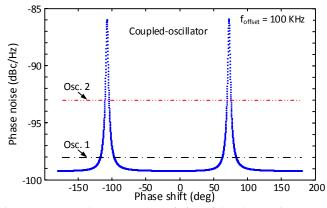
Fig. 16 Narrow pulse generator. Variation of the phase-noise spectral density at 100 KHz frequency offset obtained with the approximate formulation in (24).
