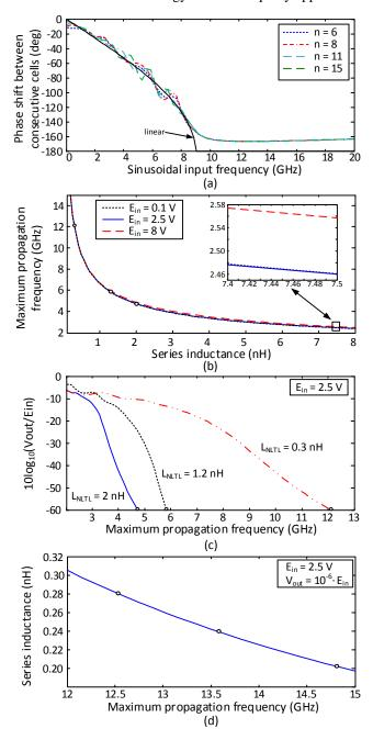
Fig. 1 Analysis of the NLTL under a sinusoidal input signal. (a) Phase shift per stage for different numbers n of NLTL cells. (b) Variation of  $f_{max}$  vs. the inductance L for different  $E_{in}$  values. (c)
