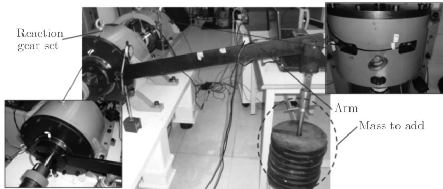
Fig. 2. Application of the external torque
