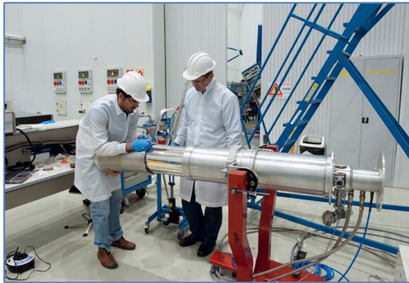
Figure 5. Assembly of the QUIJOTE test cryostat at the IAC AIV room. Sensitivities are referred to Stokes Q and U parameters.
