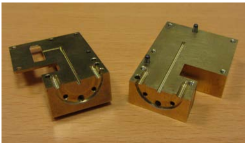
Figure 8. Photographs of the metal case (two pieces) for the patch antenna array
