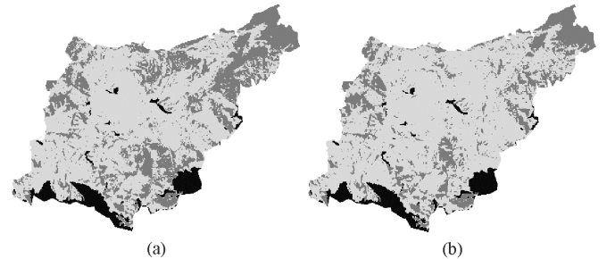
Fig. 7. Coverage maps in Gipuzkoa, considering D_{OPT}=3 and h=800 m. The covered, not covered and filtered receiving locations are depicted in light gray, dark gray and black, respectively. (a) Initial. (b) Optimized.
