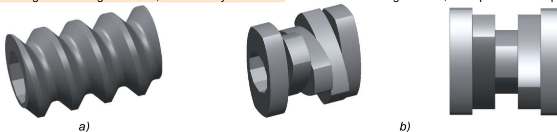
Fig. 3 – Example of screw elements: a) transport element; b) kneading module, showing the five elements and the rotation with 45° of each element
