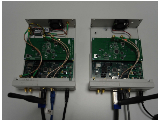
Figure 10: N210 Ettus devices with the XCVR2450 daughterboard installed. A two-antenna cognitive receiver is composed of two N210 boards connected through a MIMO cable.
