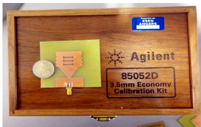
Fig .8. The fabricated antenna structure and the 3.5 mm used calibration Kit.
