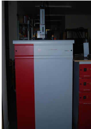
Figure 5.3: QD-MPMS XL 5T sited in the Universidad de Cantabria. All the magnetic properties of the thin films have been acquired in this equipment.
