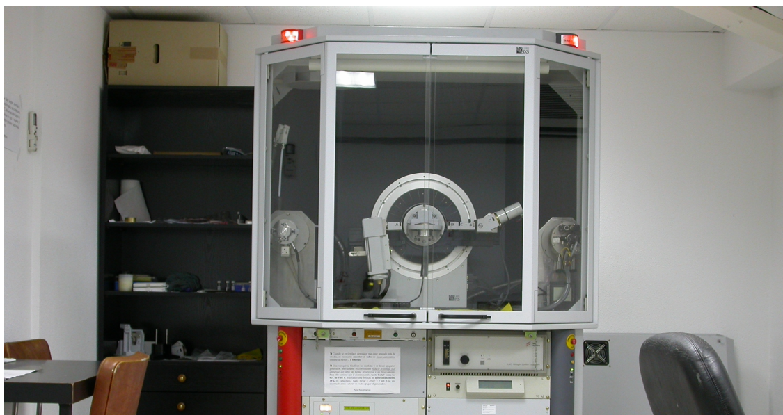
Figure 5.1: Bruker D8 Advance. It is a very flexible instrument, with several options, like changing the X-Ray tube or attaching furnaces or cryostats into the sample space.
