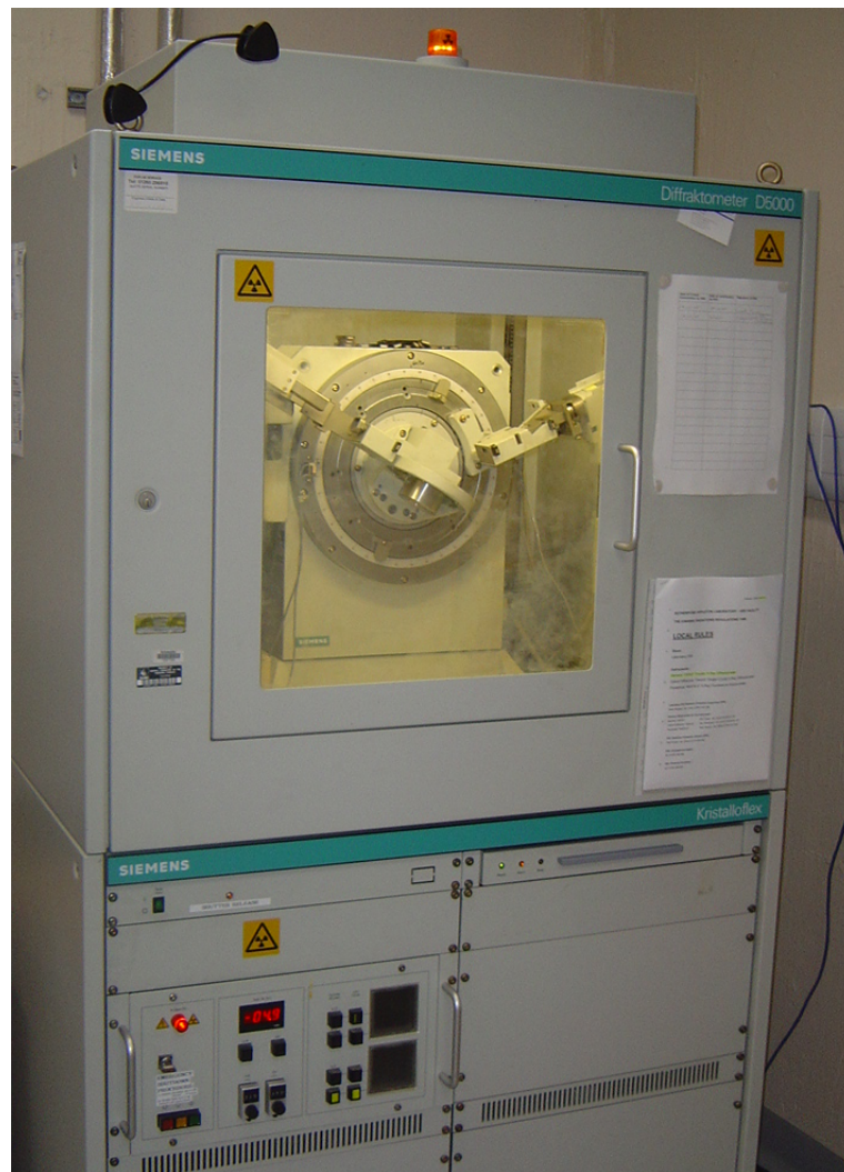
Figure 5.2: Siemens D6000 diffractometer sited in the laboratory R53 of the RAL. Its \theta/2\theta geometry is different to the Bruker apparatus.
