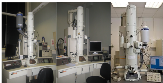
Figure 5.6: TEM used in the present study. At the left panel it is shown a JEOL 2000FX, at the middle a JEOL 2010 (both from the Imperial College, London), where at the right panel a Jeol JEM 2100 which belongs to the Universidad de Cantabria. Most of the work has been performed in the latter microscope.
