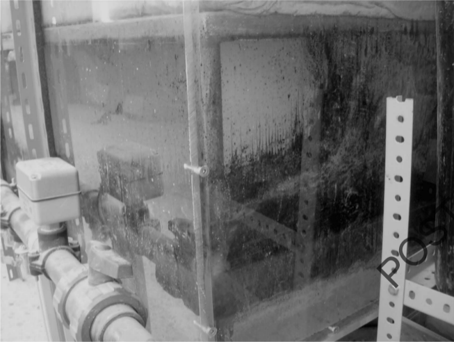
Figure 5. Oil adhesion to the SCPT inner walls.
