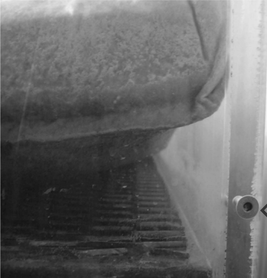
Figure 2. Filter system displacement of the SCPT after 14 rain events.
