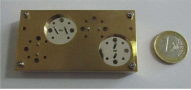
Fig. 35. Dual-band SU-8 Micromachined OMTs
