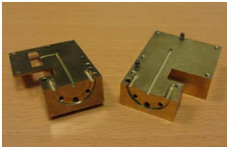
Fig.3. Photograph of the open Metal Case for the Patch Antenna Array
