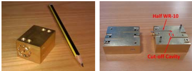
Fig.73. Photographs of the Metal Case for the Back-to-Back Transition ( 4 \times 3 \times 2.4 \text{ cm}^3 )
