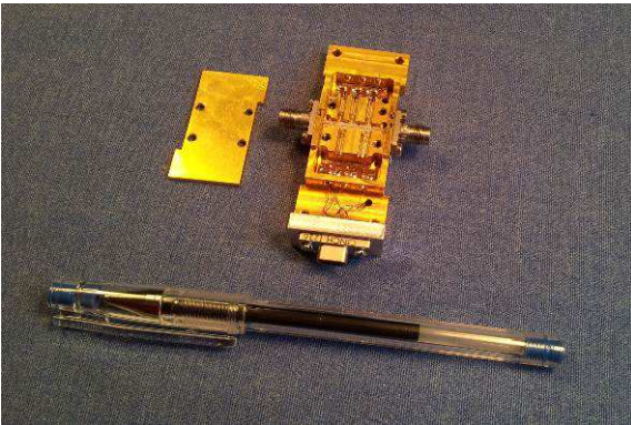
Fig. 9. LNA assembly with 2.4 mm connectors.
