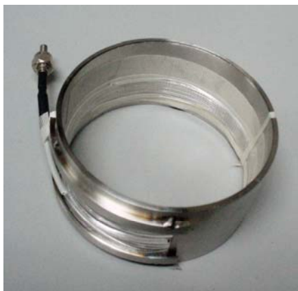
Fig.3: POF cable wound within the external section of the weld head.
