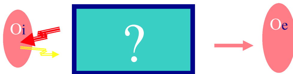
FIGURE 1 - Conceptual illustration of an Optical Sensor: Light from the object with its state information encoded in it, after travel through the optical channel, arrives the optoelectronic unit and then the decoded information, in the electrical domain, is able to be used.
