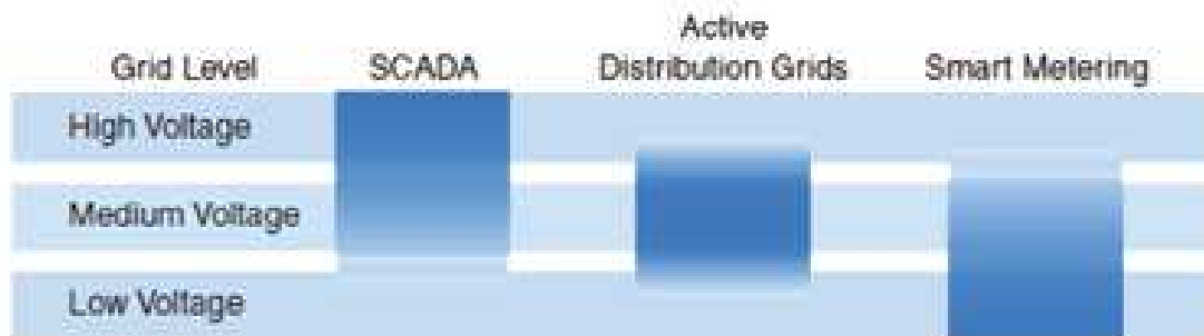
Figure 203: Common ICT applicative areas in correlation with the grid levels (Liserre et al., 2010)
