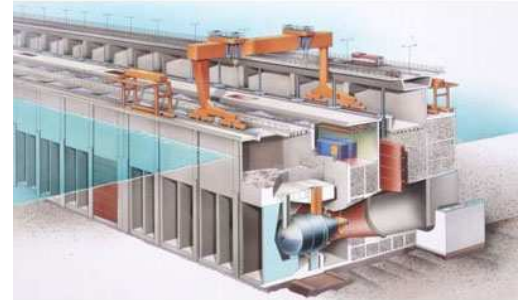
Figure 59: Tidal power plant on the estuary of the Rance River, Bretagne, France, Tidal Energy (201?)
