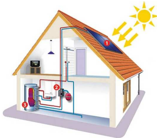
Figure 19: Domestic water heating (Harveys)
