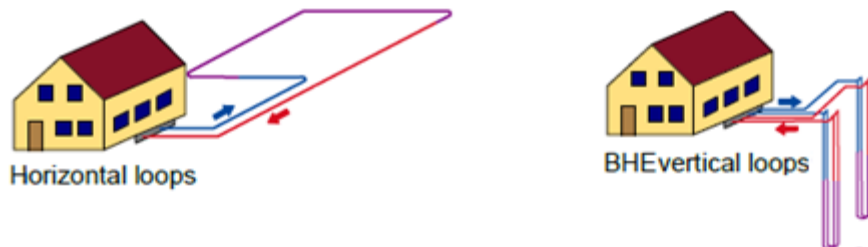
Fig E.5.5: Diagram of common ground-coupling methods (from left), horizontal and vertical loops (EGEC, 2009)
