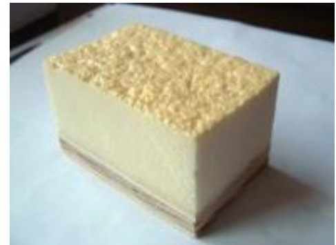
Figure EEM. 3.6: Polyurethane section (Energy Consulting, 2012)
