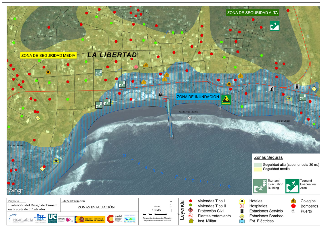
Figure 17. Evacuation areas in La Libertad area (colored areas: flooded area in blue, intermediate security areas in yellow, high security areas in green. colored dots: buildings materials).
