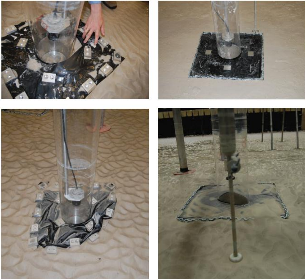
Figure 39: Scour protection with composite and rubber mat tests (Deltares, 2010)
