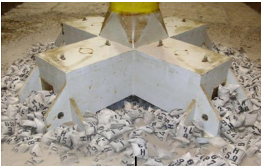
Figure 38: Scour protection hydraulic test for Strabag foundations (Mayumi Wilms, et al., 2010)
