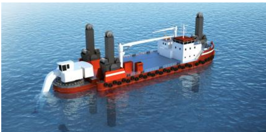
Figure 22: Back hoe on a pontoon (FKAB, 2013)
