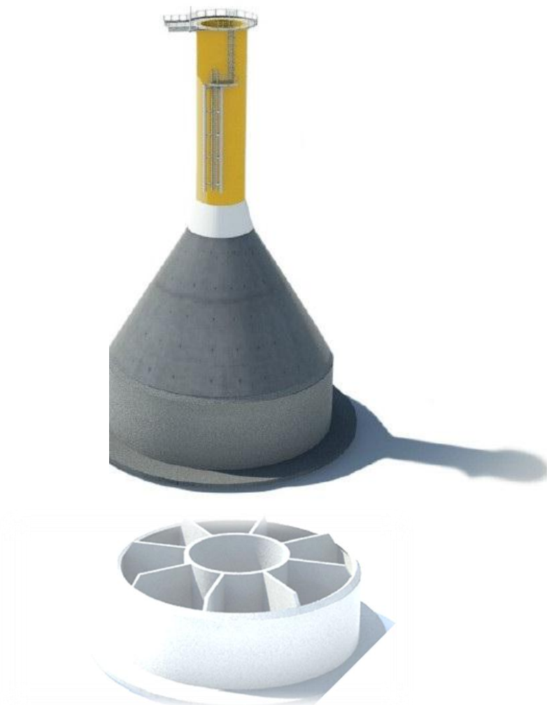
Foundation design (Gravitas)
