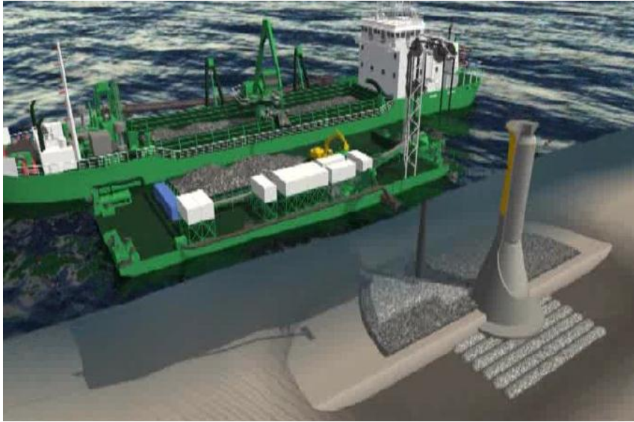
Figure 37: Scour protection in Thornton Bank (DEME, 2008)
