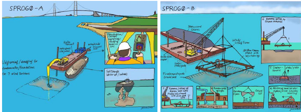
Seabed preparation (ABJV)
