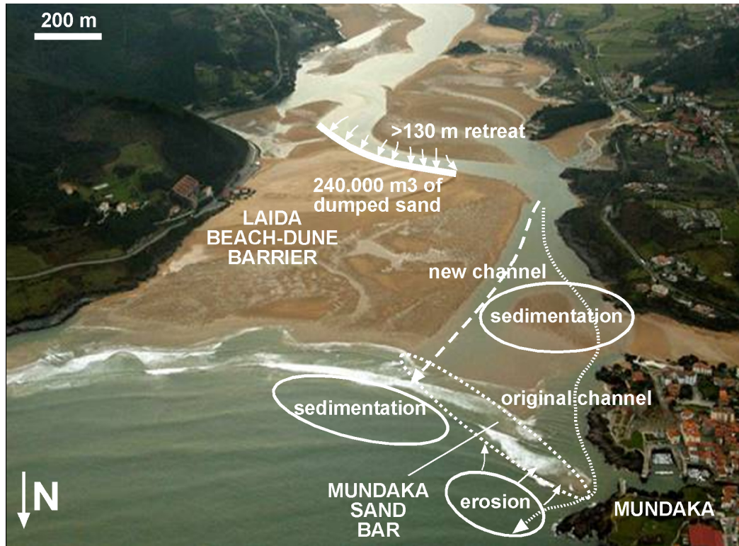
Fig. 3.- Study area and sedimentary processes involved between June 2003 (sand dumping)-May 2005 (beginning of this study).
