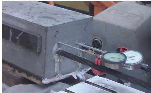
Figure 6. Placement of the transducer displacement for measuring penetration \delta .
