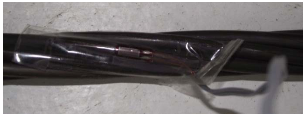
Figure 4. Placement of strain gages.
