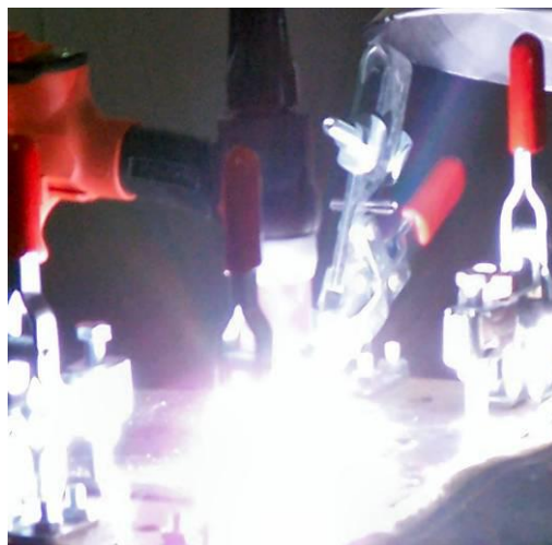
Figure 2. Plasma radiation during arc-welding test.
