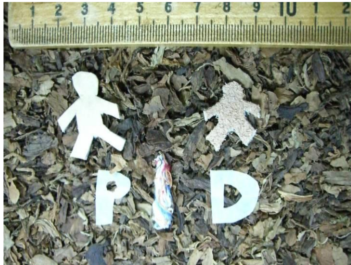
Fig. 6. Material under test: several foreign materials over chopped tobacco leaves.
