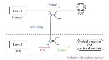
FIGURE 3: Typical configuration for a BOTDR system. FUT is the fiber under test or distributed transducer, LO is the local oscillator, and CW is the continuous wave.
