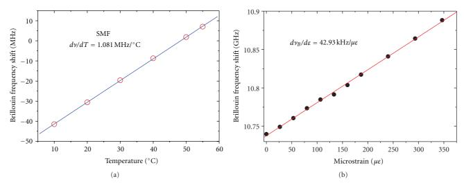
FIGURE 1: Experimental data of Brillouin shift dependence on the temperature and strain.
