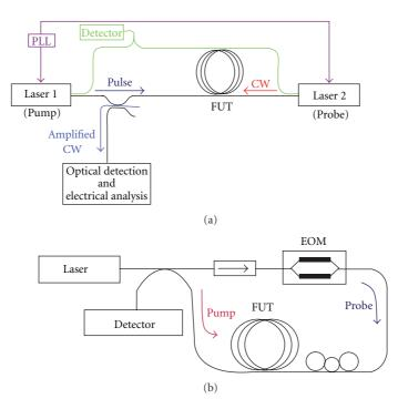
FIGURE 5: Experimental setup for BOTDA, using two sources (a) and one source (b).
