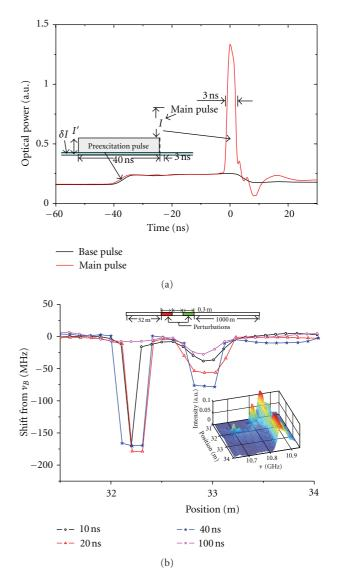
FIGURE 8: The pump light is basically formed by a pump-prepump pair pulse, and by subtracting the couple Brillouin backscattering it is possible to use larger base pulses to obtain stronger backscattered signals or to reach larger distances in the fiber. (a) Experimental data of preexcitation optical pulse. (b) Experimental data for 2 ns of main pulse and four values of P-pulse. Brillouin spectrum gain (inset figure).
