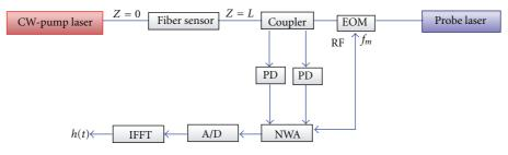
FIGURE 10: Basic schematic configuration of a BOFDA sensor system.
