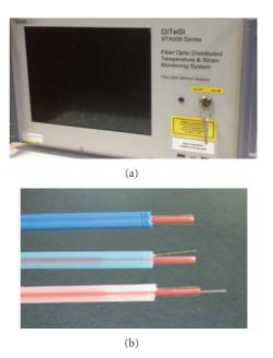
FIGURE 2: Illustration of one optoelectronic (a) and three samples of fiber transducers for both temperature and strain (b) of a stimulated Brillouin distributed sensing system, courtesy of the Photonic Engineering Group of the University of Cantabria.
