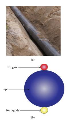
FIGURE 16: Illustration of a pipeline in a buried process (a). Scheme of the distributed fiber transducer placement with respect to the pipe section (b).
