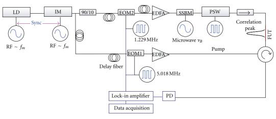
FIGURE 9: Experimental setup for BOCDA technique.
