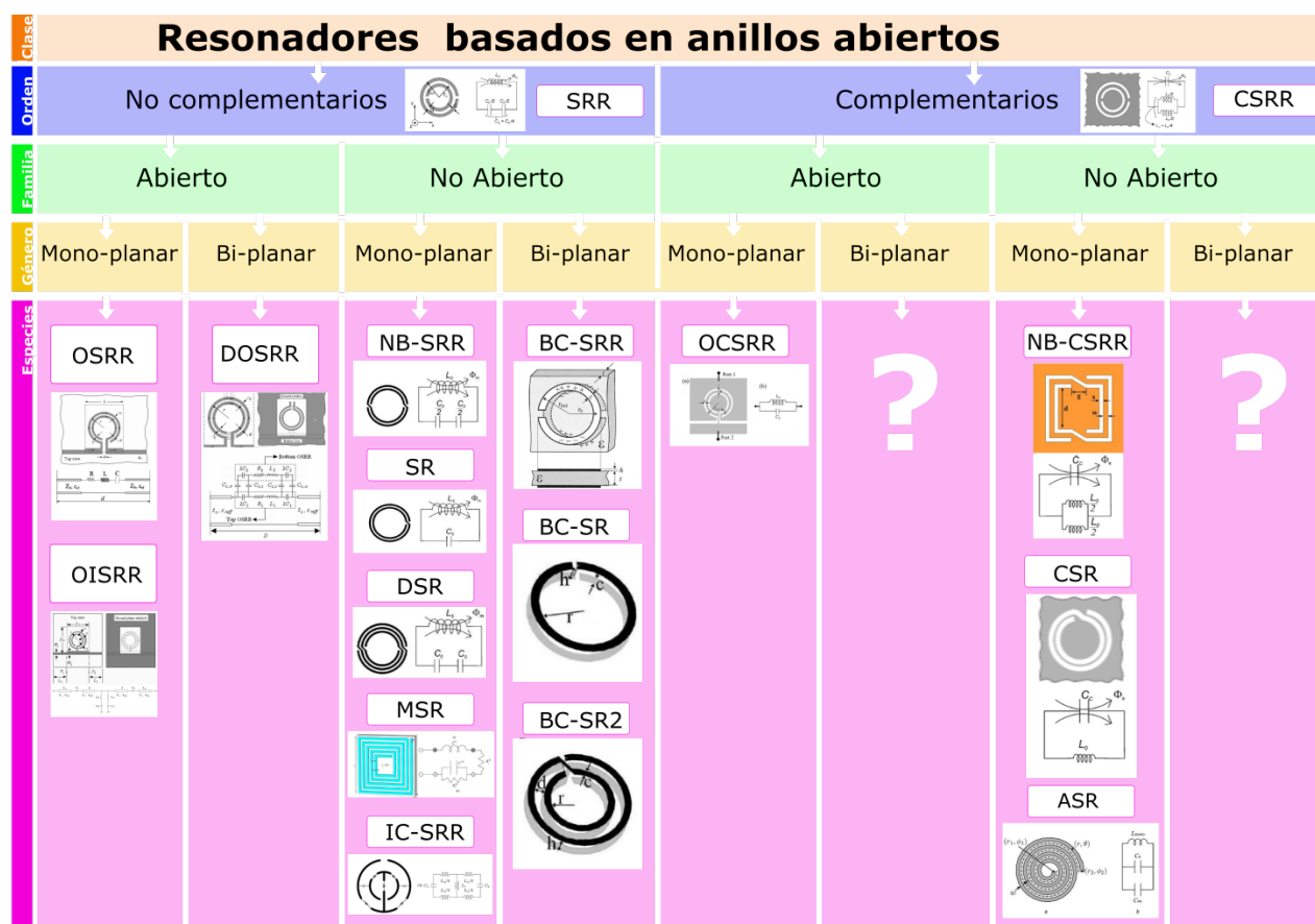
Figura 2.11: Taxonomía lineana propuesta para celdas basadas en resonadores de anillos abiertos. Las figuras se han extraído de: SRR, CSRR, NB-SRR ( Nonbianisotropic Split Ring Resonator ), SR ( Spiral Resonator ), DSRR ( Double-slit Split Ring Resonator ) de [85]; OSRR ( Open Split Ring Resonator ) de [14]; MSR ( Multiple Split Ring Resonator ) de [86], ICSRR ( Inductively Connected Split Ring Resonator ) de [87]; BC-SRR ( Broadside Couple Split Ring Resonator ) de [88]; BC-SR ( Broadside Couple Spiral Resonator ) y BC-SR2 ( Broadside Couple Two Spiral Resonator ) de [89]; OCSRR ( Open Complementary Split Ring Resonator ) de [15]; NB-CSRR ( Nonbianisotropic Complementary Split Ring Resonator ) de [90]; CSR ( Complementary Spiral Resonator ) de [91] y ASR ( Archimedean Split Resonator ) de [92].
