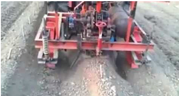
Figure 1 Cassava vertical planting machine.
