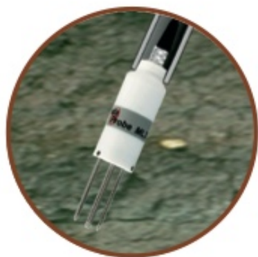
Figure 3. Installation of Theta probes at an angle of 20 degrees.
