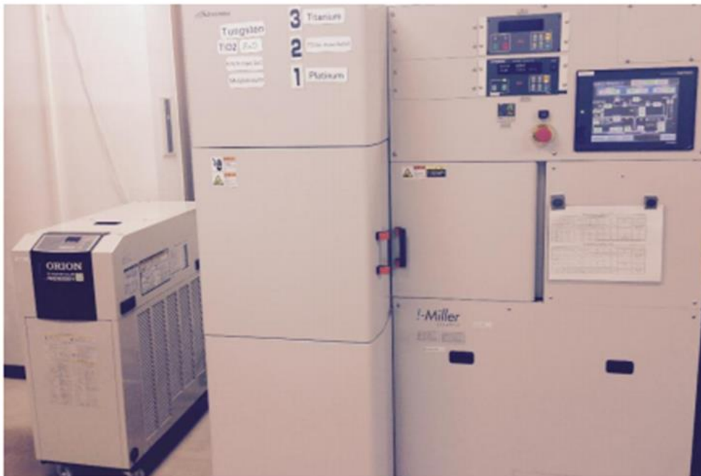
Figure 2.9 The set-up for metal deposition. Three targets are equipped with this sputtering system.
