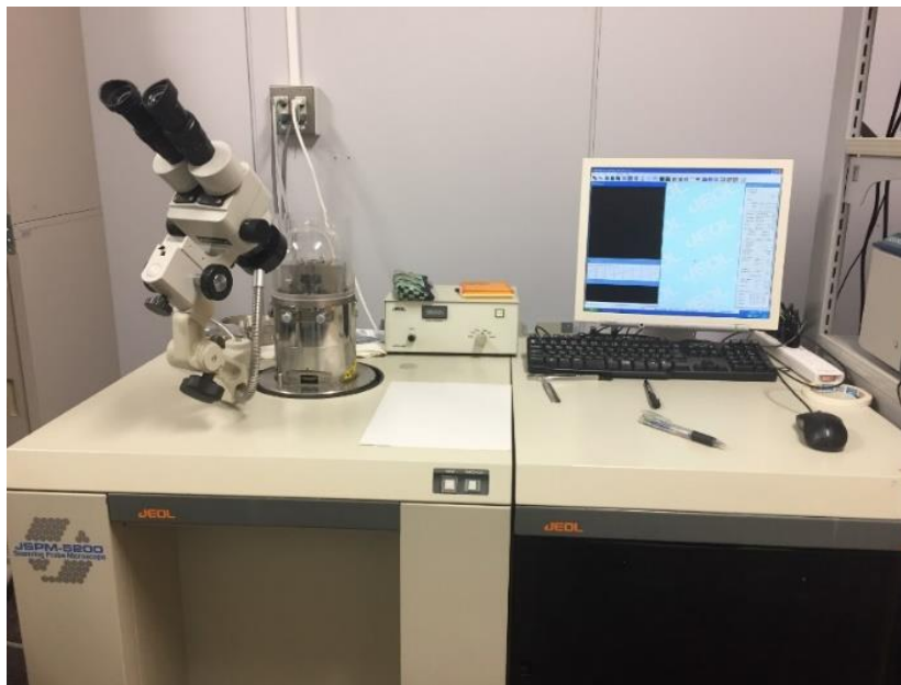
Figure 2.10 The AFM setup and software used to control the AFM (JEOL measurement) equipment.
