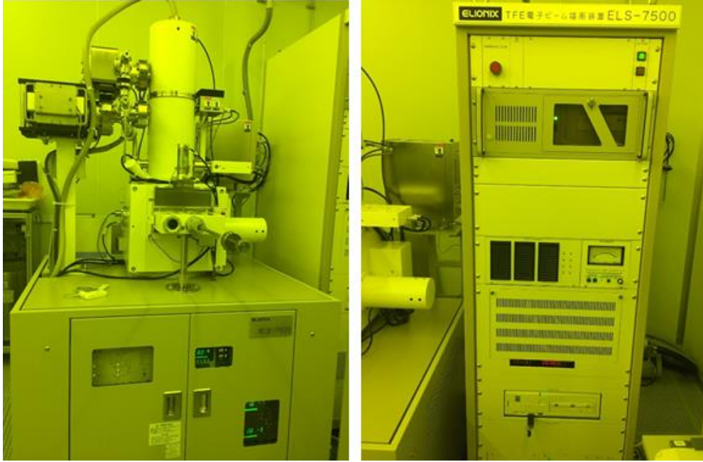
Figure 2.7 EB-lithography system used in this experiment for drawing the pattern, equipped with the control panel (right) controlled by a computer interface.
