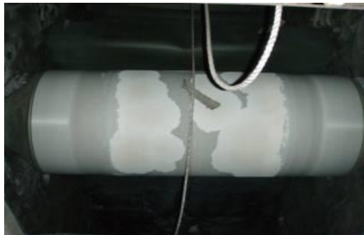
Fig. 1.7 Hearth roll used in continuous annealing furnace for producing steel sheet
