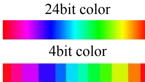
Fig.4. 3 The change of color bit (24bit -> 4bit)
