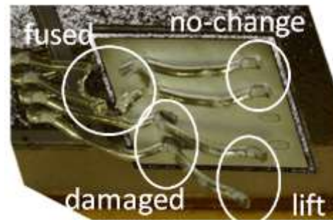
Fig. 3. Failed specimen diode after 4677 cycles. This photograph was flipped upside down to adjust orientation of following SAT images.
