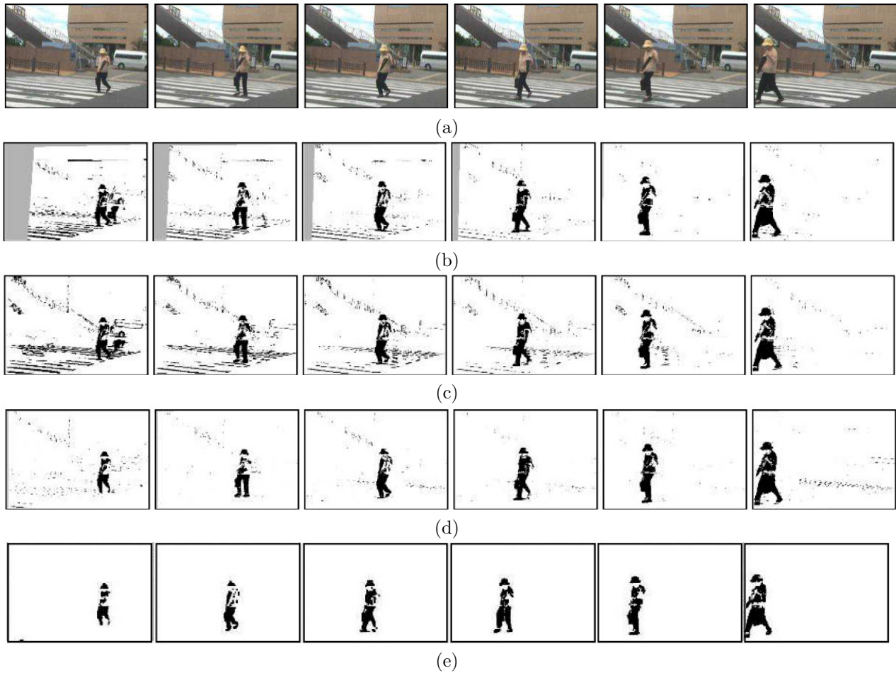
Fig.5: Comparison of the Proposed Background Estimation Technique with Other Techniques. Experimental Results on Turning-left Video which Consists of 98 Frames of 320 \times 220 pixels. (a) Part of the Original Frames, (b) The Result Obtained from the Temporal Median (TM) Method, (c) The Result Obtained from the Running Average (RA) Method, (d) The Result Obtained from the Proposed Technique Employing the Normal Distribution Model (NM). (e) The Result after Applying Expansion-Contraction Post-processing to (d)
