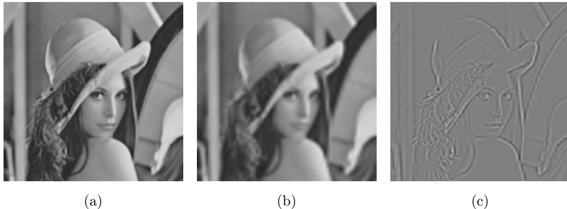
Fig. 1. Image blurring property in Lena. (a) A given image I , (b) LPF image I_l , (c) HPF image I_h .
