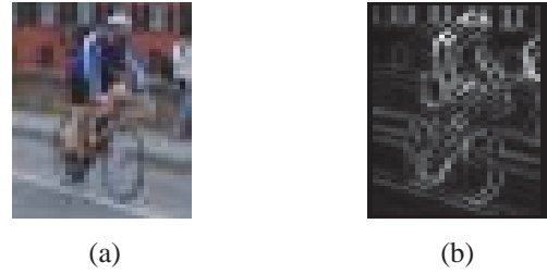
Fig. 2. A processed bicycle image: (a) An original image, and (b) its oriented gradients image.
