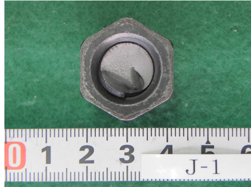
(a) \alpha=0 (fatigue life 151,860 cycles)
