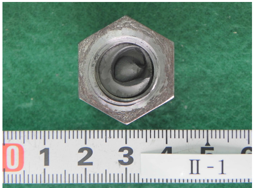
(b) \alpha=\alpha_{\text{small}} (fatigue life 242,810 cycles)
