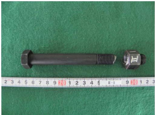
(b) \alpha=\alpha_{\text{small}} (fatigue life 242,810 cycles)
