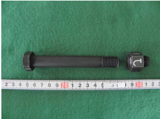
(a) \alpha=0 (fatigue life 151,860 cycles)
