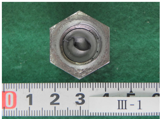
(c) \alpha=\alpha_{\text{middle}} (fatigue life 184,770 cycles)
