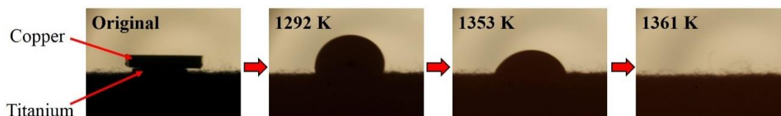
Figure 5.2.2 Representative photographs of wetting process of Cu-10 mass % Ti alloy on carbon fiber felt in the placement state C with increasing the heating temperature
