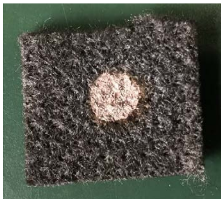
Figure 5.2.3 Photographs of Cu-10 mass % Ti alloy on carbon fiber felt after wetting experiment (frontal view)
