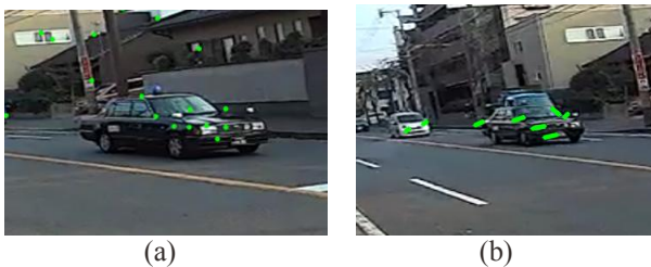
Fig. 2 Example of motion vectors detection on a vehicle: (a) Detected feature points, (b) detected motion vectors.
