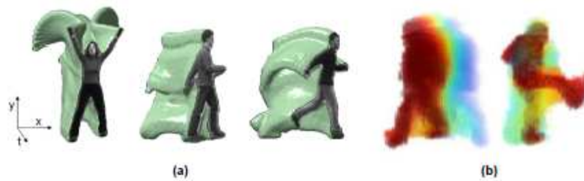
Fig. 2.1 Various motion representation schemes. (a) Space-time volume of stacked silhouettes [55, 84], (b) Motion history volumes [79]. (a) is viewed from a single camera, whereas (b) shows a recency function over reconstructed 3-D voxel models.
