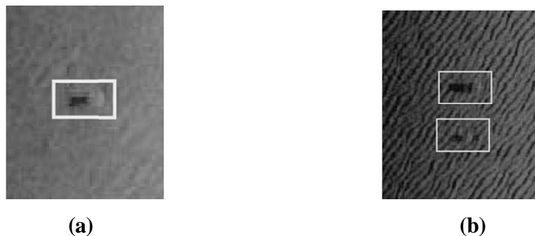
Figure 3-12. Detection results for seabed objects on the mud flat board and the sandy area board: (a) Seabed object on the mud, (b) seabed object on the sandy bottom.
