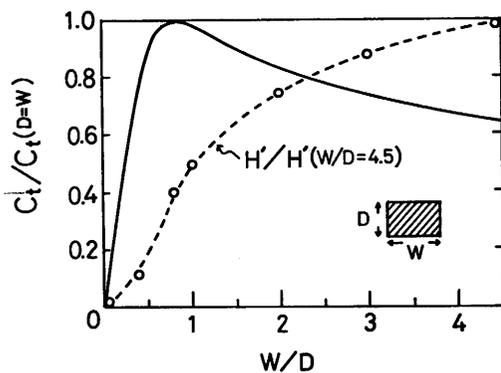
Fig. 4. Fiber cross sectional shape effect on capturing capacity.
