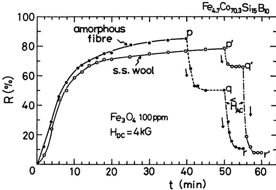
Fig. 1. Experimental results of HGMS for  $\text{Fe}_3\text{O}_4$  using stainless steel wool (s. s. wool ; white circles) and amorphous fiber (black circles) : real lines show the capturing process, and dotted and chained lines show the flushing processes without and with modulated AC fields, respectively.
