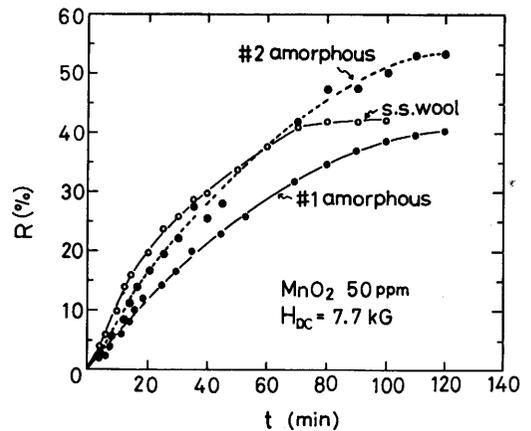
Fig. 3. Experimental results of HGMS for  $\text{MnO}_2$  using s.s. wool and two kinds of amorphous fibers with cross-sectional shapes of 125-25  $\mu\text{m}$  at #1 and 65-50  $\mu\text{m}$  at #2.
