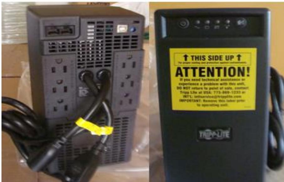
**Figura 15 UPS (Uninterruptible Power Supply).**
