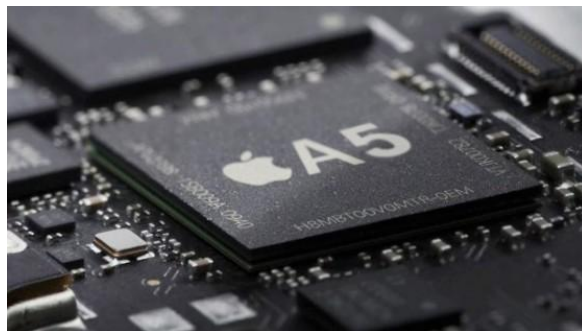
Fig. 0.22 Apple A5 Processor (Apple)
