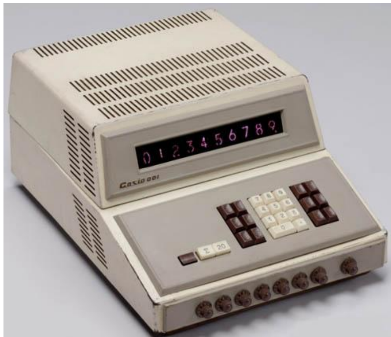
Fig. 0.1 First compact 100% electronic calculator ( www.kirianet.com )
