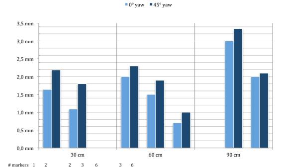
**Figure 7:** Co-registration error measured according to number of markers detected, user-markers distance and off-plane angle
