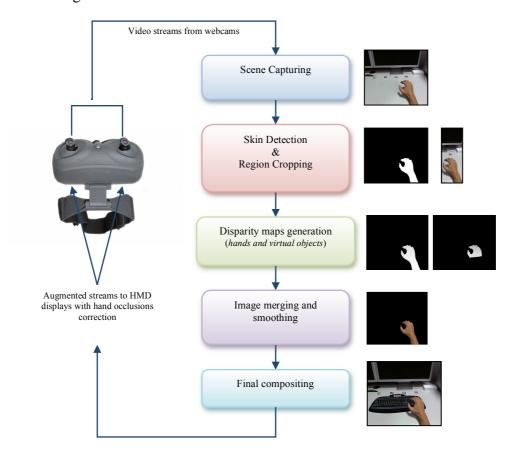
Fig. 13. The overall architecture of the approach proposed.
