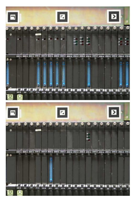
**Figure 8:** Original frame (top) and diminished view (bottom). Only the required elements are left visible, while textured polygons hide potentially confusing items.
