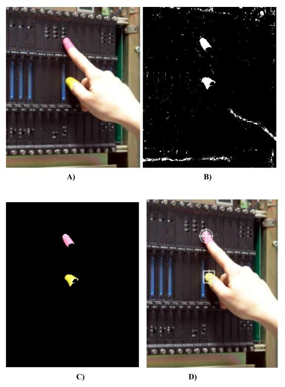
**Figure 4** – Fingertips tracking in four steps: (A) original frame grabbed from the camera; (B) candidate pixels highlighted (C); matching regions found; (D) resulting tracking
