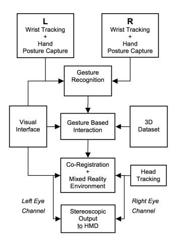
**Figure 18**. A schematic view of the whole architecture.
