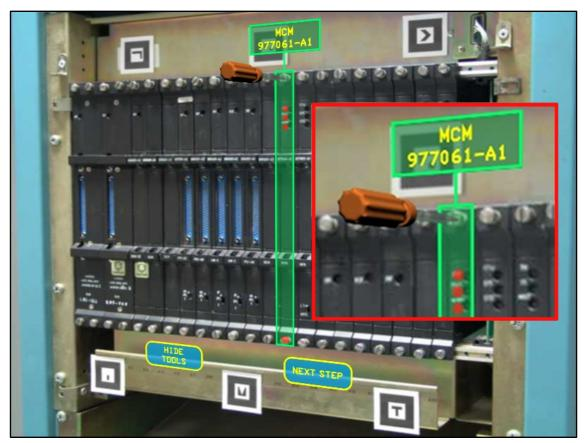
**Figure 3:** Panel augmented by virtual labels, tools and GUI (inset) a magnified view showing the small amount of co-registration error
