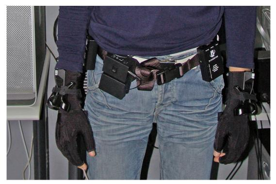
**Figure 19.** Wireless instrumented gloves (Data Glove 14 ultra from 5DT) coupled with wrists/head wireless motion tracking (IS-900/VET Inertial Tracking from Intersense ) worn during testing.
