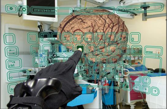
**Figure 23**. Sample images of the user's field of view (simulated) during gesture interaction within the mixed reality environment. The floating interface layout (which can be hidden (top) or shown (bottom) via a gesture toggle) is projected onto the central region of the field of view to enable the selection of the required functionalities as well as the interaction with virtual objects.
