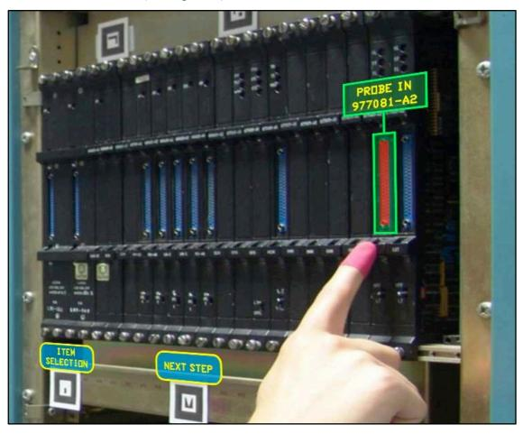
**Figure 5:** User interacting with the servicing assistance environment through a contactless finger based interface while performing a simulated maintenance procedure.
