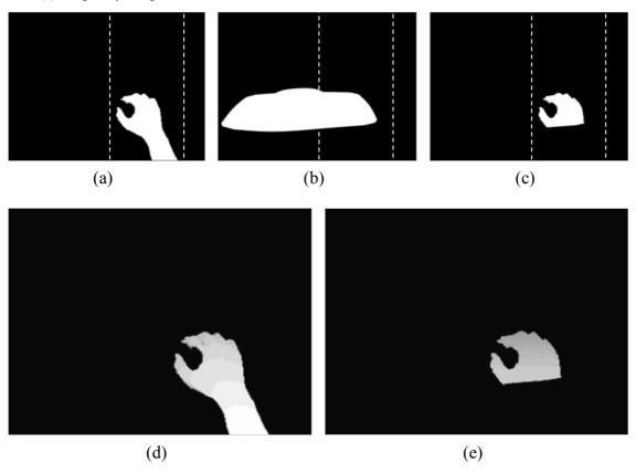
**Fig. 15.** Skin detection with closure functions refinement (a). Alpha channel of augmented objects rendered onto the video stream (b). Disparity map of user's hand segmented from the scene by the skin color-based detection (d). Disparity map of the crop of the region where augmented virtual contents overlap the hand (e).
