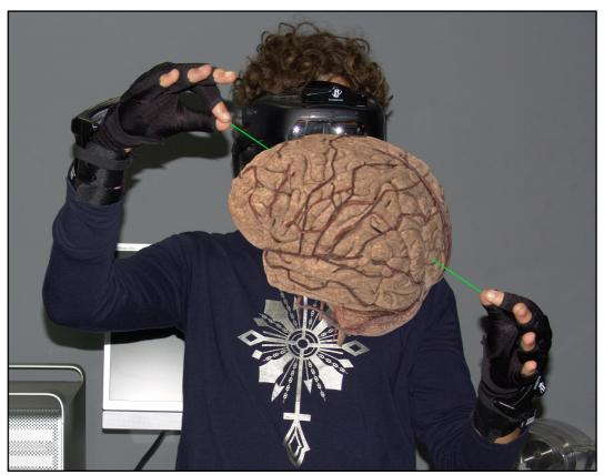
**Figure 24**. User performing object rotation by means of two virtual handles, corresponding to the extremities of the green vector. This image shows the scene from the point of view of a third person, and is obviously simulated, due to the optical see-through design of the HMD. The brain model is the result of a true medical imaging processed to generate a 3D geometry, and further optimized (about 625,000 triangles). The shown color texture is fictional.
