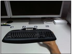
**Figure 12.** Left: A virtual model of a keyboard rendered onto a captured frame of real environment to augment it. The hand positioned along the right side of the keyboard does not ruins the Mixed Reality illusion. Right: The same MR scene, but as the hand is positioned over the keyboard, it is occluded by the virtual content.
