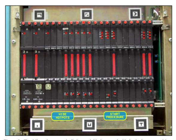
**Figure 2:** The full marker set and all the available hotspots highlighted after successful coregistration calibration.
