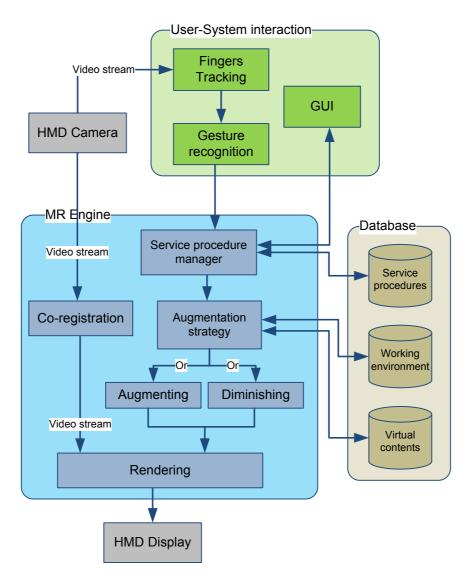
**Figure 1:** *The overall schematic view of the system.*
