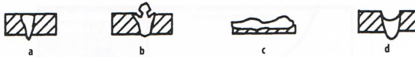
Figure 2.10 Range of weld shapes varying usually with speed: a normal/good; b undercut; c humping (longitudinal section); d drop out.
