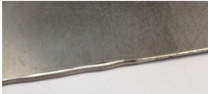
Figure 6.6 Edge joint of Inconel 625 without oxidation
