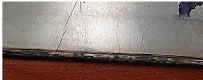
Figure 6.4 Oxidation level of the Inconel 625 in preliminary tests
