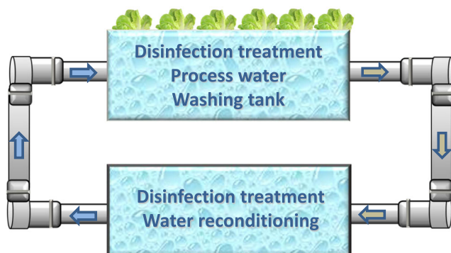
Fig. 1 Schematic representation of the water disinfection treatments applied in a fresh-cut processing line to treat process water within the washing tank, which is in contact with fresh produce, and for water reconditioning of process water that can be reused in the washing tank
