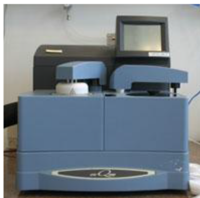
Figure 3.3 : Differential scanning calorimetry (DSC, TA Q1000).
