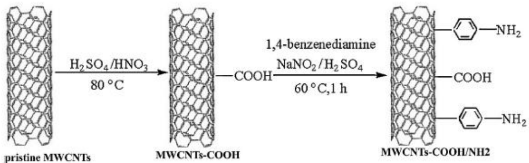
Figure 2.3 : Functionalization of CNTs with carboxyl or amine groups.
