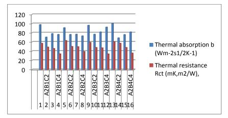
**Figure 5.12:** Histogram of thermal absorptivity and thermal resistance values of layers with common outer shell A2 or PBI gold with 200 g/ m<sup>2</sup>.
