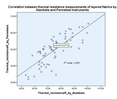
Figure 5.9: Correlations between thermal resistance measurements of layered fabrics by Alambeta and Permetest.
