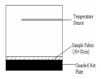
Figure 3.6: Guarded hot plate apparatus[28].
