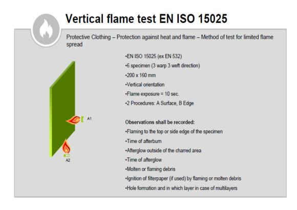
Figure 3.2: Vertical flame test exemplary according to EN ISO 15025 [83].
