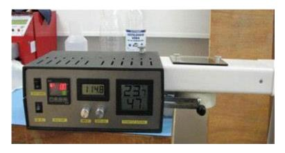
Figure 3.8: Photograph of Permetest test instrument[29].
