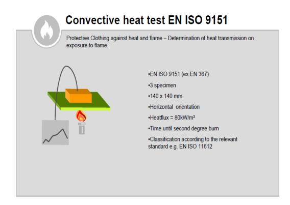
Figure 3.3: Convective heat test according to EN ISO 9151 [83].
