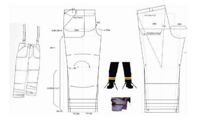
Figure 2.2: Construction and design of the protective trousers [61].
