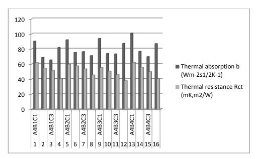
Figure 5.16: Histogram of thermal absorptivity and thermal resistance values of layers with common outer shell A4 or Nomex Outershell Tough Ripstop with 195 g/ m<sup>2</sup>.
