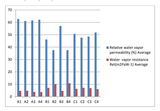
Figure 5.2: Histogram of relative water vapor permeability and water vapor resistance of single layer fabrics.
