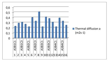
**Figure 5.15:** Histogram of thermal diffusion values of layered fabrics with common outershell A3 or PBI Matrix with 200 g/ m<sup>2</sup>.
