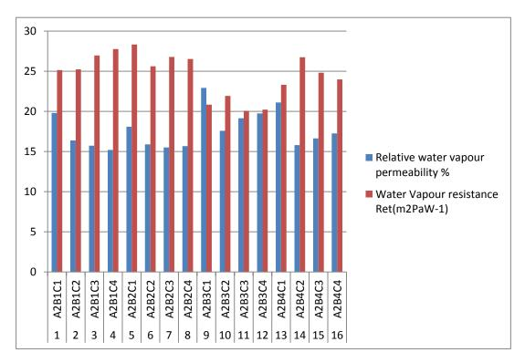
**Figure 5.4:** Histogram of multilayered fabrics water vapor resistance when outer shell A2 is common.
