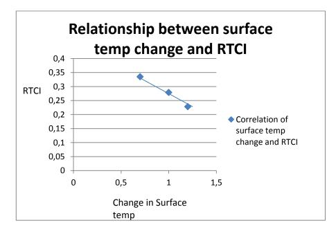
Figure 5.30: Relationship between the values of RTCI and change in surface temperature of fire fighters protective clothings.
