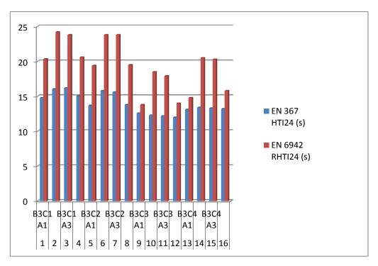
**Figure 5.22:** Histogram of layered fabrics EN367 HTI 24 and EN6942 RHTI 24 results with common moisture barrier B3or PU membrane laminated to knitted fabric with 85 g/m<sup>2</sup>.
