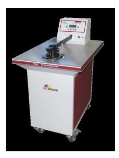
Figure 3.10: Air permeability tester[30].
