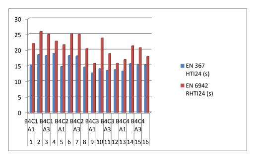
**Figure 5.23:** Histogram of layered fabrics EN367 HTI 24 and EN6942 RHTI 24 results with common moisture barrier B4 or PU membrane laminated to knitted fabric with 145 g/m<sup>2</sup>.
