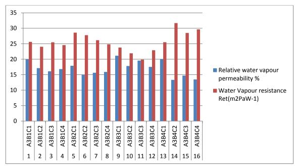
Figure 5.5: Histogram of multilayered fabrics water vapor resistance when outer shell A3 is common.
