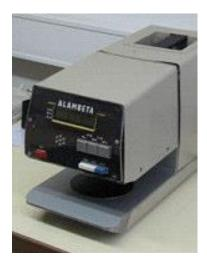
Figure 4.3: Alambeta instrument .
