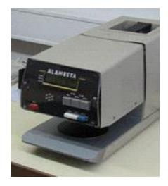
Figure 3.7: Photograph of Alambeta test instrument[27].
