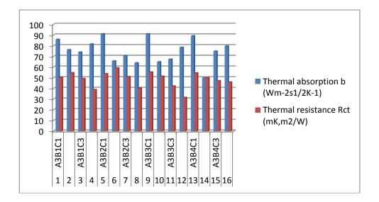
**Figure 5.14:** Histogram of thermal absorptivity and thermal resistance values of layers with common outer shell A3 or PBI Matrix with 200 g/ m<sup>2</sup>.
