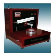
Figure 4.1: Prowhite air permeability tester.
