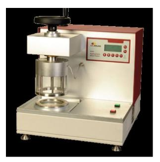
Figure 3.9: Photograph of hydrostatic head tester[30].
