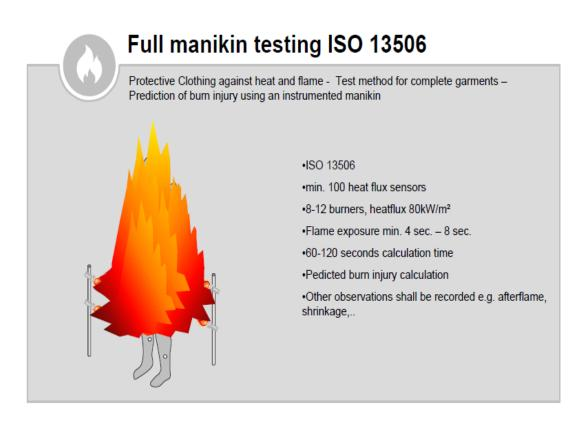
Figure 3.4: Full manikin testing exemplary according to ISO 1350 [83].
