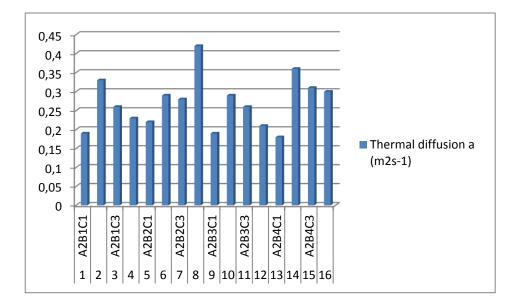
**Figure 5.13:** Histogram of thermal diffusion values of layered fabrics with common outershell A2 or PBI gold with 200 g/ m<sup>2</sup>.
