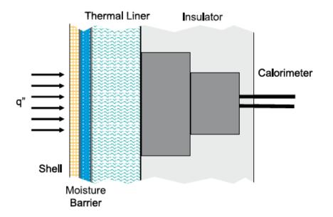
Figure 1.3: Measuring heat transfer in turnout systems[21].
