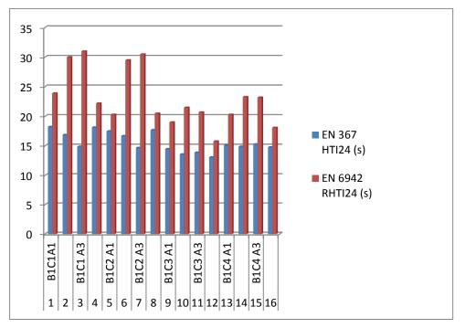
**Figure 5.20:** Histogram of layered fabrics EN367 HTI 24 and EN6942 RHTI 24 results with common moisture barrier B1 or PU membrane laminated to nonwoven (50/25/25) with 55g/m<sup>2</sup>.
